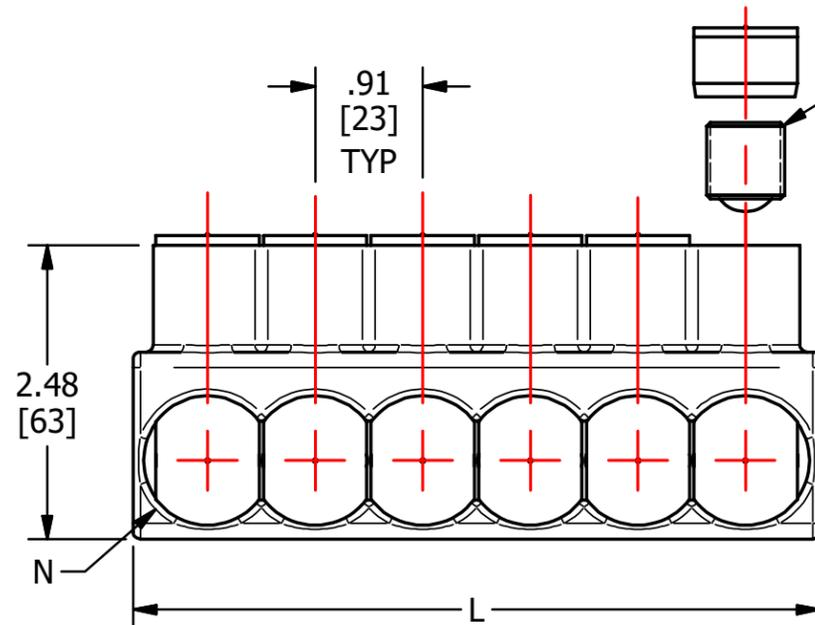
SCREWS ARE SUPPLIED WITH CONNECTOR AND COMES FULLY ASSEMBLED.
